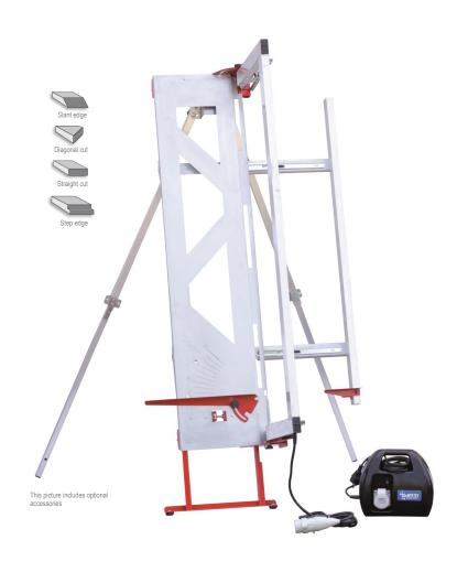
Ideal for cutting polystyrene (EPS, XPS) insulation panels.
